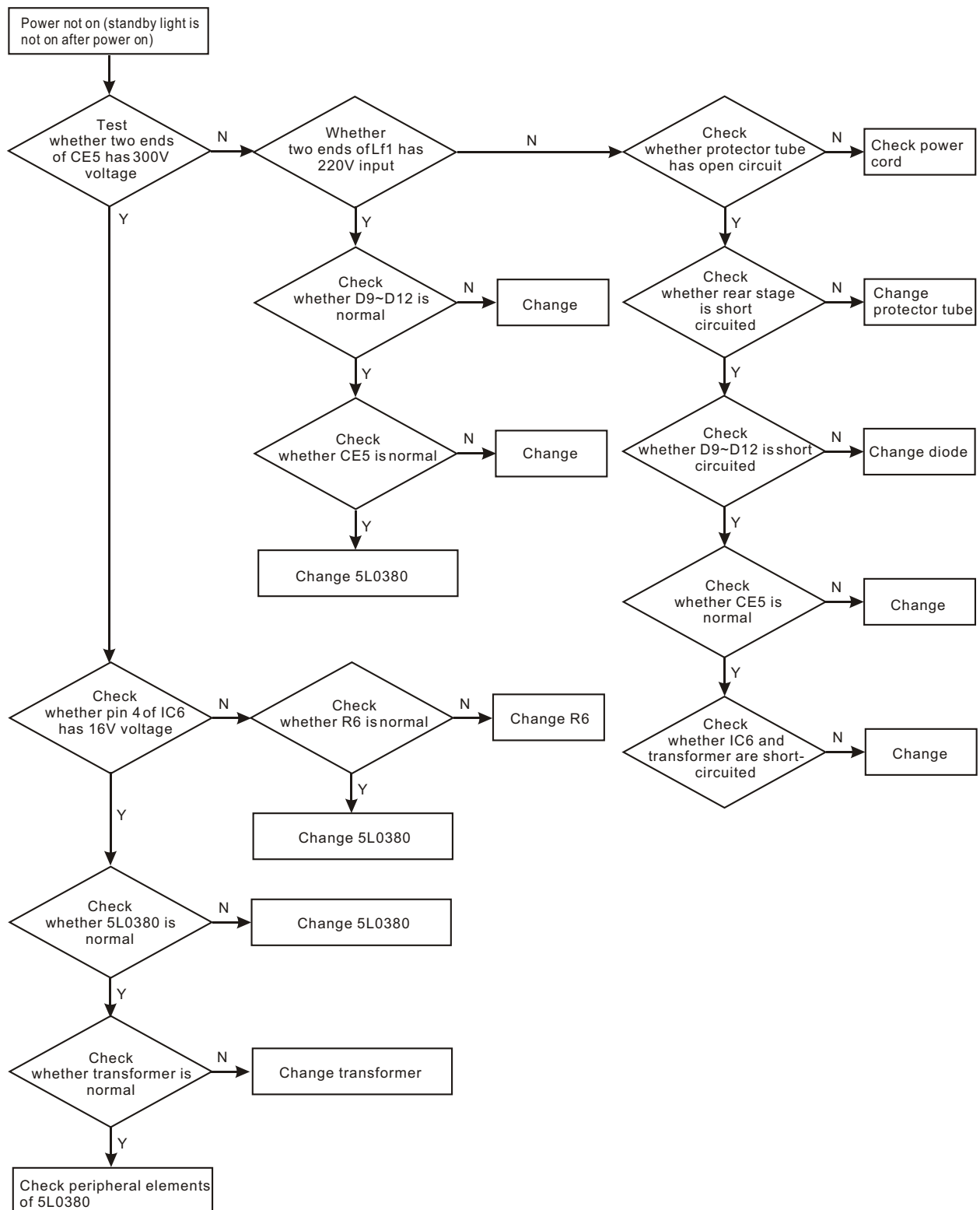
Figure 3.3.2.3 Troubleshooting flow chart for “Power not on”
